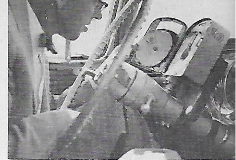
Dr. Jim Fogo equips test car with a tachometer chart for recording time, speed and acceleration
